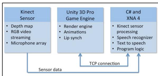
Figure 3. High-level architecture of the software-hardware interfaces and feature handling.
